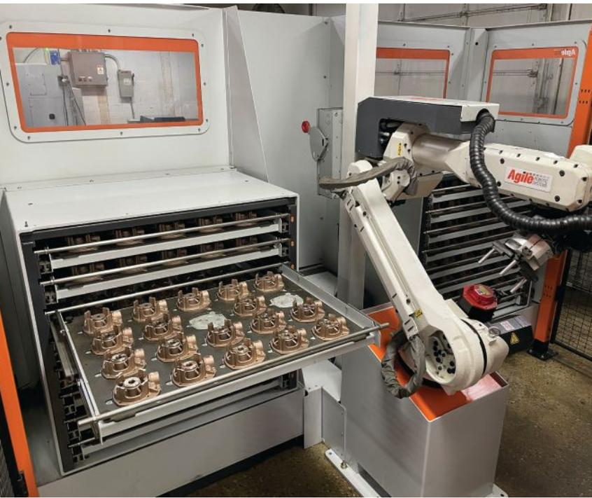
MTH Pumps achieves lights-out automation overnight through pairing its 12 Mazak Integrexes with auto-loading gantries. One Integrex is also paired with a machine-tending robot from Agile Robotic Systems, and the combination of machine-tending robot and gantry loader extends this machine's unattended operations over the weekend.
