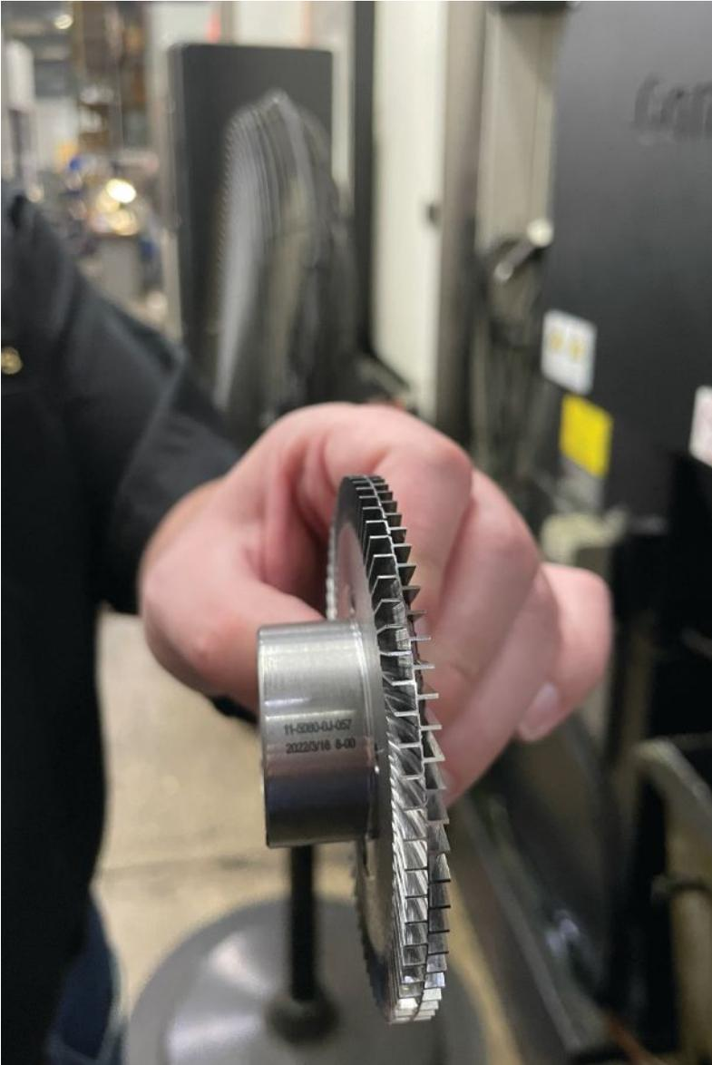
“The impeller is the heart of the pump,” Tremain says. But the impeller’s ubiquity doesn’t make its 0.0005-inch perpendicularity and parallelism tolerances any simpler to machine, especially at a thickness of 0.082-inch. The Integrex machines must mill vanes on each side separately without disrupting the perpendicularity-parallelism tolerance relationship.
